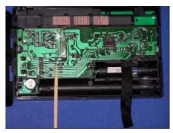
(where the coils meet the plastic slot), it is unlikely to salvage the loopstick intact in one piece, but for purposes of the transplant modification, the empty plastic slot will provide a convenient routing space for the new 40/44 Litz wires, without the stray inductance that would occur if the stock loopstick were left in the cabinet.
