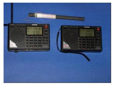
loopstick, but it will also use a 40/44 Litz wire coil found to have the optimal inductance match (with the 4734 DSP chip varactor) for maximum AM sensitivity. In detailed testing with an 81-turn Slider coil and this 7.5" Amidon ferrite bar (shown in the picture to the left), AM signal strength readings were checked on the PL-380's digital display for different coil positions (and different inductances) as the coil was slid across the ferrite bar.
