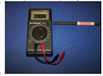
554 µh inductance was found to be optimal for a loopstick constructed of a 40/44 Litz wire coil on a 7.5" type 61 ferrite bar in the PL-380 model, recent testing indicates that the changing any of the experimental parameters (ferrite bar size or length, ferrite mix, Litz wire type, coil "Q" or DSP radio model) may result in a different optimal inductance value..
